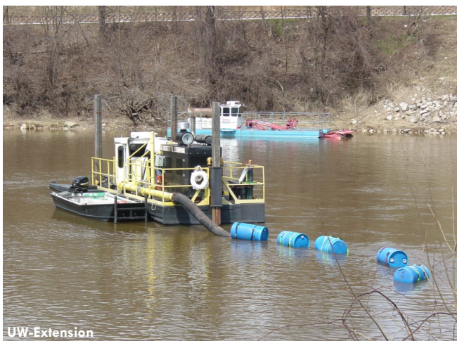
A hydraulic dredge at work in the lower river Superfund cleanup of PCB-contaminated sediment. Watch for it again summer, 2012.
