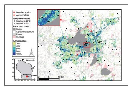
A network of 150 sensors provided temperature and humidity measurements for both urban and nonurban areas around Madison, WI. The upper-left box magnifies Madison's most extreme heat island, its densely populated isthmus, and shows how much of the area is covered with impervious, urban surfaces.
