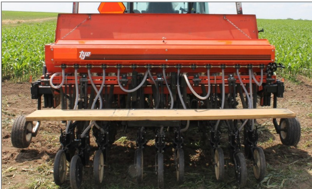
Figure 1. Modified grain drill to allow seeding into corn.
