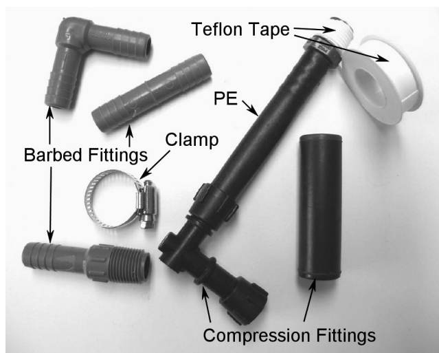
Figure 6. Examples of barbed and compression fittings, clamp, and Teflon tape.
