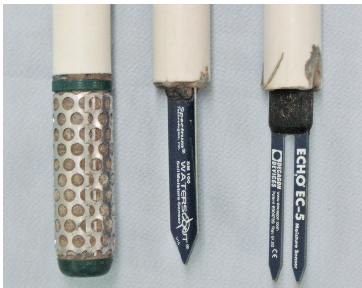
Figure 13 Stationary sensors mounted in the end of a ½-inch PVC pipe
