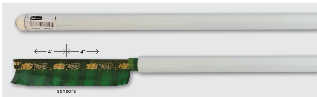
Multi-depth capacitance soil moisture sensor in PVC pipe
