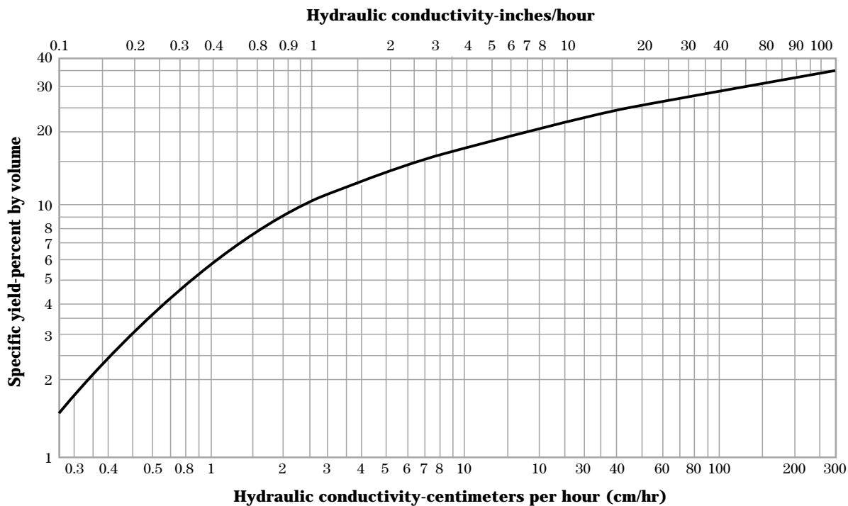
Figure 3 Curve showing general relationship between specific yield and hydraulic conductivity
