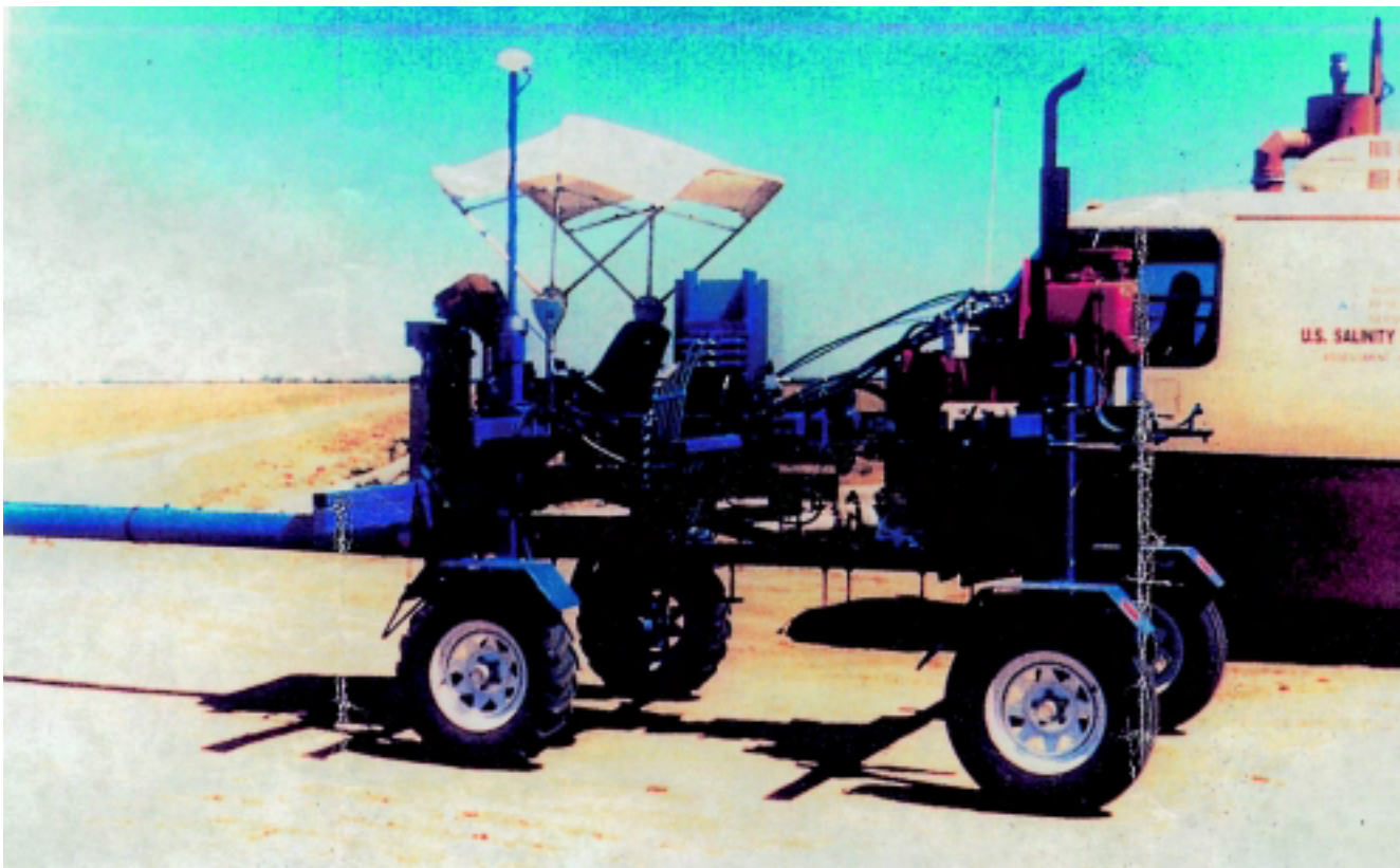
Figure 2 Combination, mobile electromagnetic-induction/four-electrode sensing system
