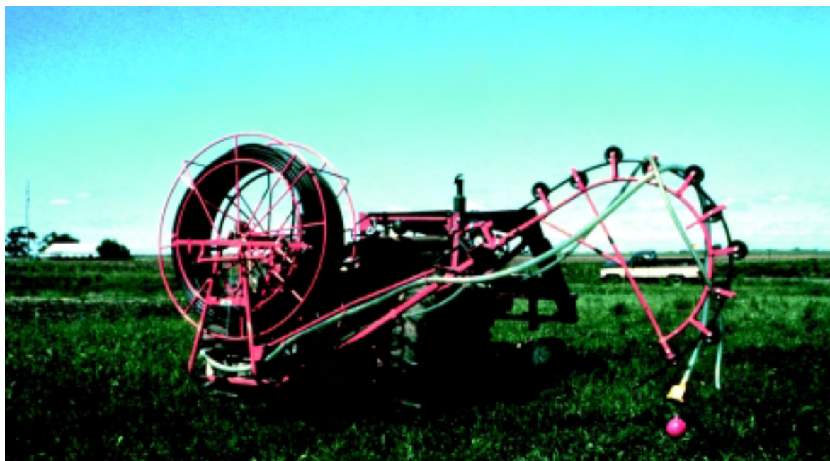
Figure 14-48 High pressure jet cleaning
