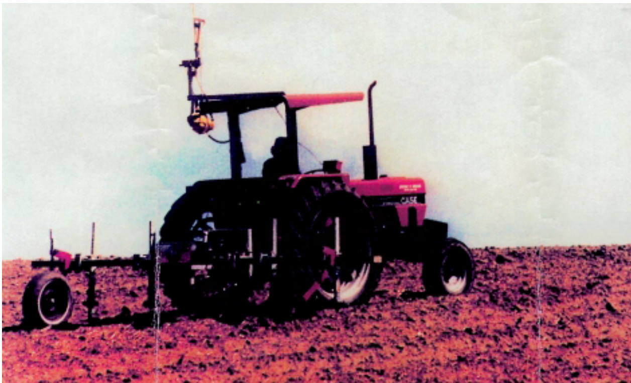
Figure 1 Mobile four-electrode sensing system
