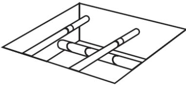
*Maintain minimum clearance. Cross at an angle as close to 90 degrees as possible.*
