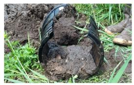
Figure 5: Evident sediment buildup in a tile line during a repair to a blowout in Eastern WI
