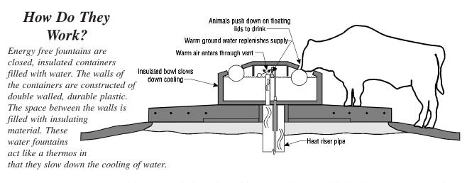
Energy free fountains use available heat (called geo-thermal heat) from the ground, below the frost line. Ground water enters the fountain through a float valve assembly at ground temperature, usually about 45°F (7°C). Ground water acts as the fountain's heat source. The water slowly cools, but as an animal drinks from the fountain, warmer ground water replenishes the fountain. This continual exchange of warm water for cold provides heat to offset the effects of cooling.
