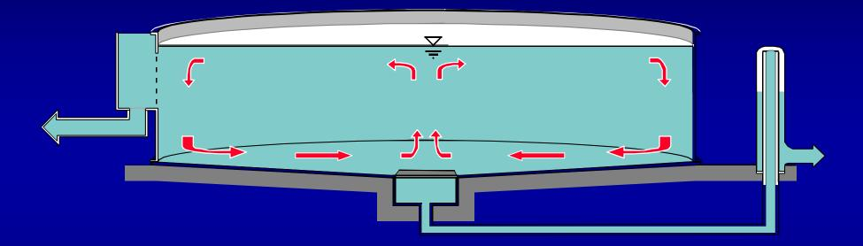
Primary rotating flow creates secondary radial flow:
