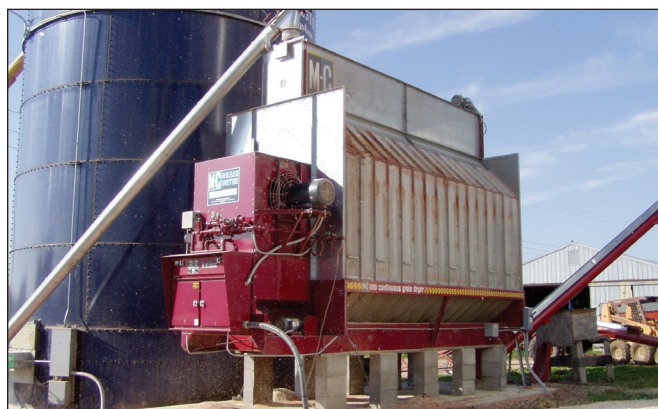
Figure 1: Horizontal cross-flow dryer. Source: Scott Sanford
