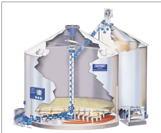
Figure 5: In-bin continuous-flow dryer with internal recirculation / discharge auger. Source: Shivvers
