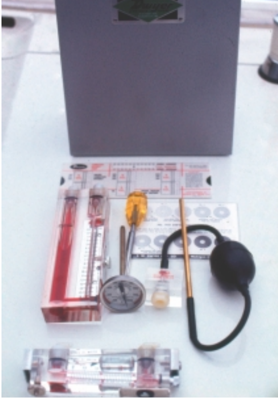
Top: If you have more than five heating units, a $300 combustion test kit will pay for itself in improved fuel efficiency; Right: Locate thermostats and sensors in an aspirated box in the plant zone.
