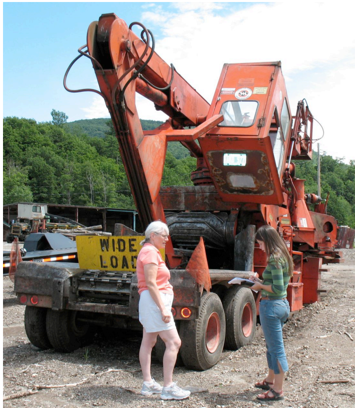
This Morbark chipper, owned by Lathrop's, can chip boles of up to 27 inches and can cost up to $480,000.
