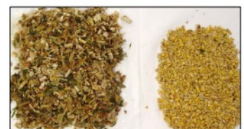
Figure 5. Example of separated stover and kernel fractions using the water separation technique.
