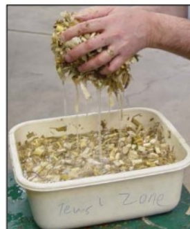
Figure 3. Skimming and removing the floating stover.
