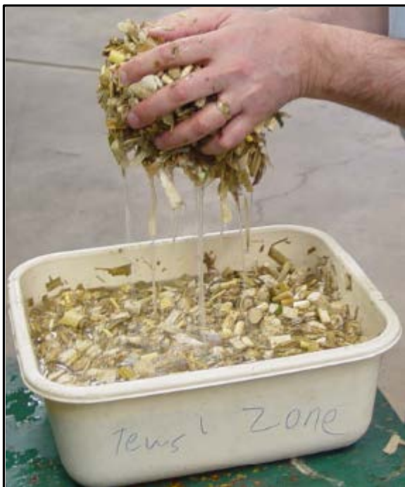
Figure 3. Skimming and removing the floating stover.
