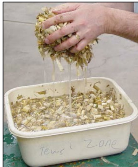
Figure 3. Skimming and removing the floating stover.
