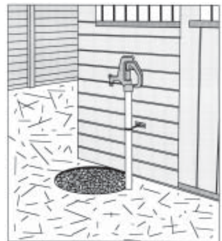
Figure 2. Design detail for freezing conditions, such as this self-draining water hydrant, will be needed in most horse stables.
