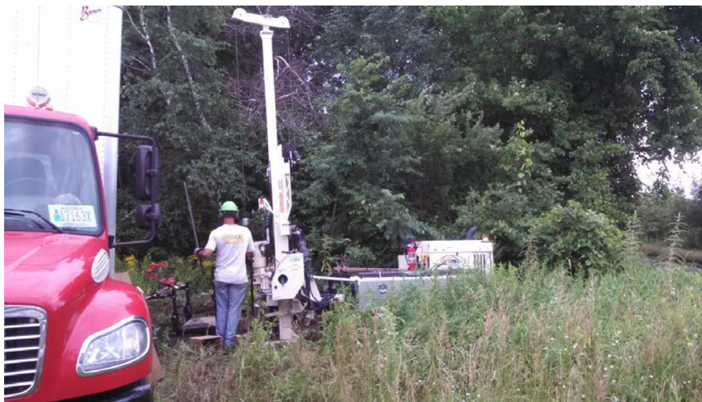
Figure 3. Geoprobe drilling near the river.
