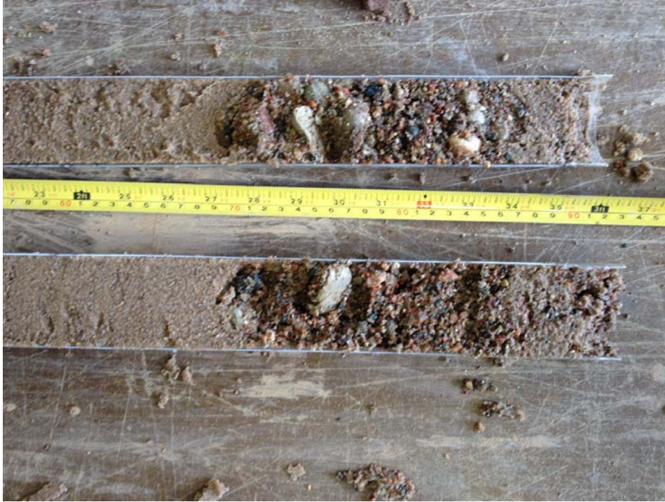
Figure 4. Typical Geoprobe core being examined.
