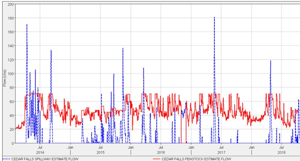
Figure 12. Estimated discharge from Cedar Falls Dam separated into penstock discharge (red) and tainter gate discharge (blue).
