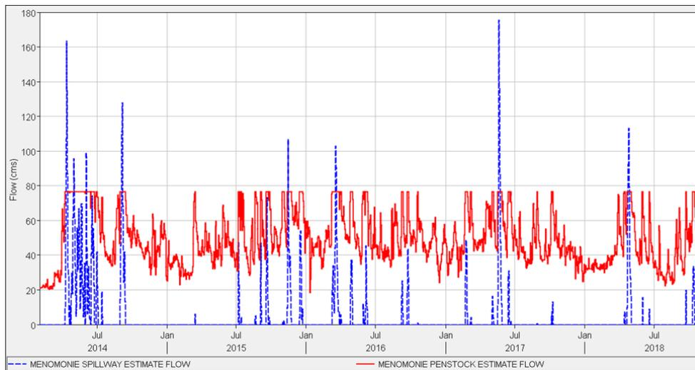
Figure 13. Estimated discharge from Menomonie Dam separated into penstock discharge (red) and tainter gate discharge (blue).
