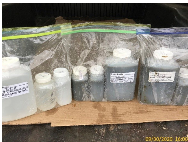
Photo 17: From left to right, comparison of water samples taken above the confluence, in the manure flow path, and where the flow path met the stream
