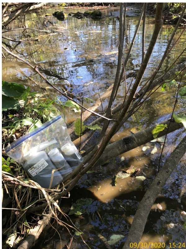
Photo 16: Water samples taken where manure entered Sandy Creek. E. coli result in this sample was 259,000/100ml, total nitrogen was 184 mg/L, and total phosphorus was 46 mg/L
