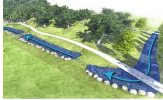
Stormwater Swale System
