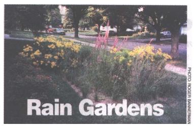
Rain gardens are designed to absorb stormwarer runoff from surfaces such as roofs) driveway's and parking lots. As such they should be 10 to 15 feet away from buildings where runoff natlurally flows toward the garden instead of toward the basement. "I predict that in less than 10 years, rain gardens will be required in all new home construction to keep storm water runoff on the property," Watts said.
